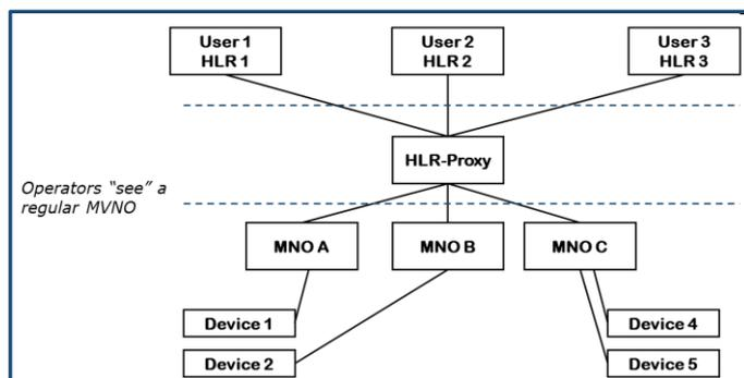
**Figure 2** The use of an intermediate, independent ‘HLR-proxy’ allows the operators to ‘see’ a regular MVNO, while there can be multiple parties, each with a sub-IMSI range in their own HLR, behind this proxy.
